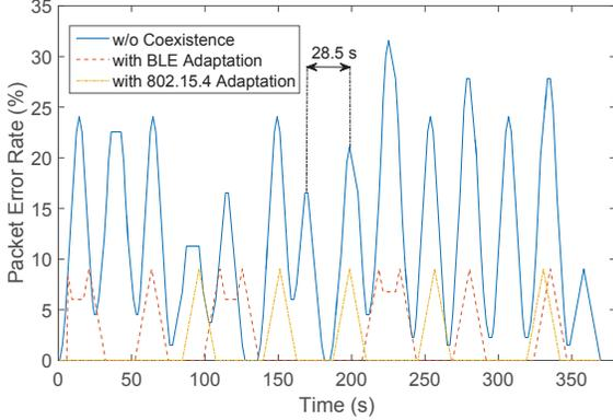
Fig. 10. PER of BLE links over time in two-channel experiments
