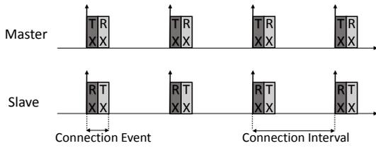
Fig. 2. Time-domain structure of communications in BLE
