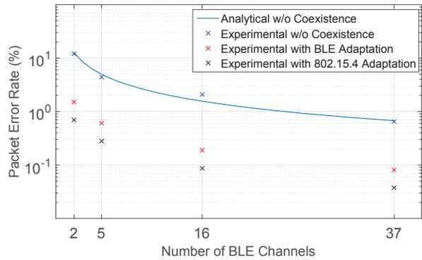
Fig. 8. PER of BLE Links for analytical and experimental results
