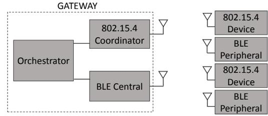
Fig. 4. Network structure for cooperative coexistence solution
