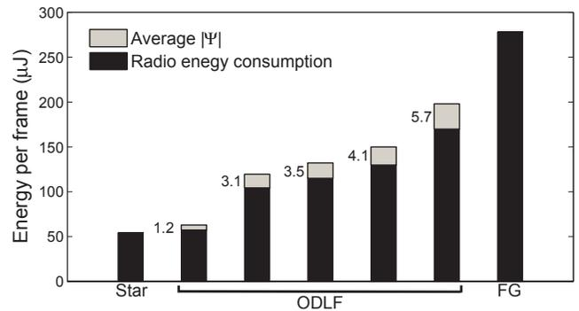
Fig. 10. Average energy consumption using ODLF protocol in experiments with different link quality, and the consumption in Star and FG protocols.
